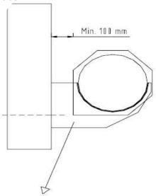
Mount the fan either horizontally or vertically in a weather-protected location.
