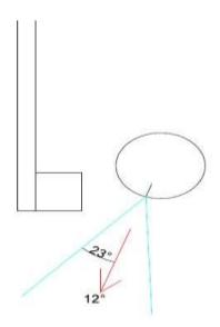
In exposed and critical applications, protect the area between the wall and the air curtain to prevent heat or cooling leakage.
