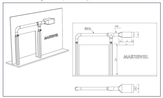
AS 50K Horizontal air curtain, water-battery, filter box and connection box.
